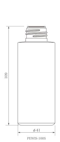
Bottle material: PET  $Molding\ method\ \vdots\ Injection\ stretch$ blow molding
